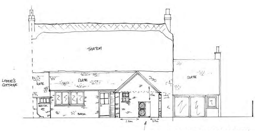
Proposed Air Source Heat Pump location within opensided car port to rear of building to minimise visual impact on listed building, minimise sound impact on neighbours and meet building regulation and manufacturer siting requirements. See photos, block plan for additional details.
